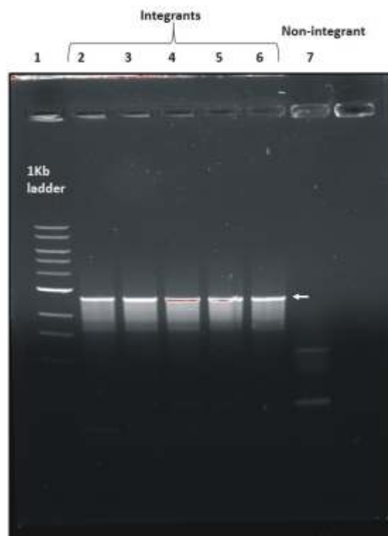
Fig. 1: PCR based screening of possible integrants (Lanes 2-6). Lane 7 is negative control (nonintegrated yeast genomic DNA)
