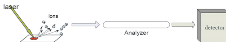
Fig.2 Scheme graph of MALDI-TOF MS
