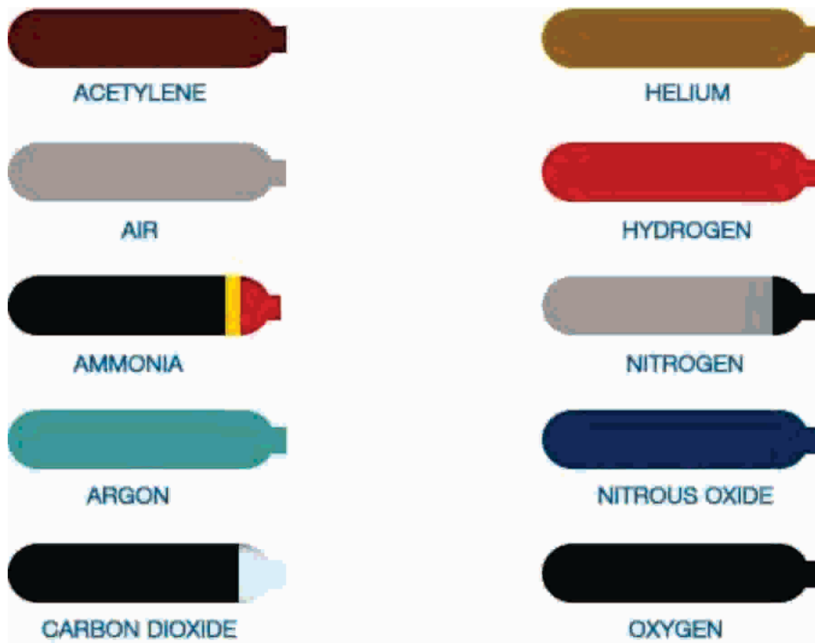
Colour-coded gas cylinders in use
